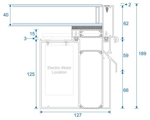
Please note that the electric motor shown here is for illustrative purposes and is not binding in technical detailing and sizing.
